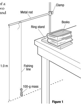
release the mass. Measure the time that the pendulum takes to make 20 complete back-and-forth swings. Record this time in Data Table 1. Also make note of the speed with which the pendulum swings back and forth.
